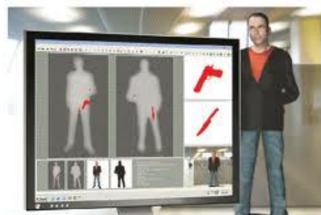
1. Passive millimeter-wave imaging can reveal weapons that are concealed under clothing.
